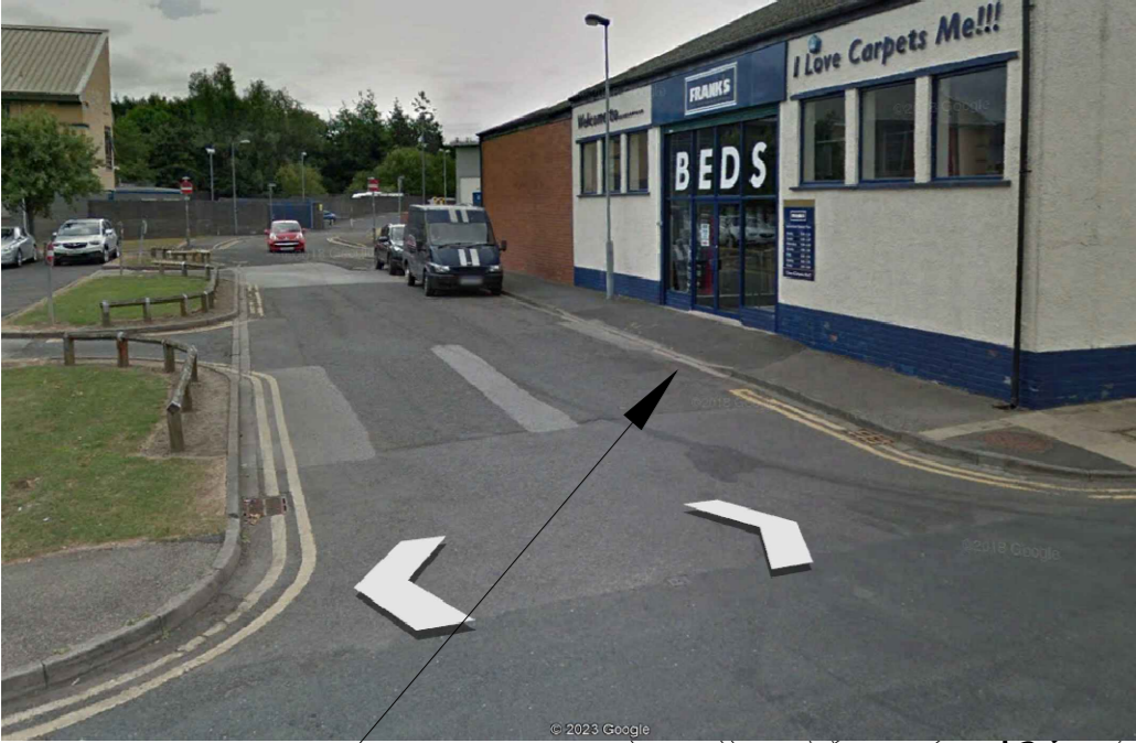
Proposed temp. double yellow linesto front of Franks Flooring so site vehicles can pass (i.e. crane / wagons etc.)
